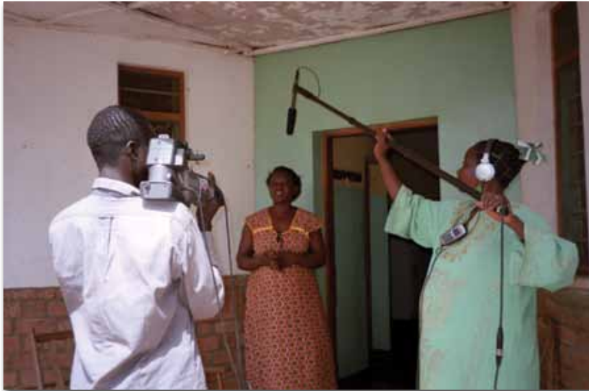
Directional microphones provide high-quality sound. They can be mounted on a boompole (as shown), used with a handheld grip, or mounted directly on certain cameras. (Southern Sudan, 2007)
